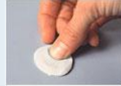
3. Apply to repair surface within 10 minutes.
